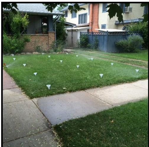
Example of "catch can" test, the most crucial step in the physical lawn auditing process.
